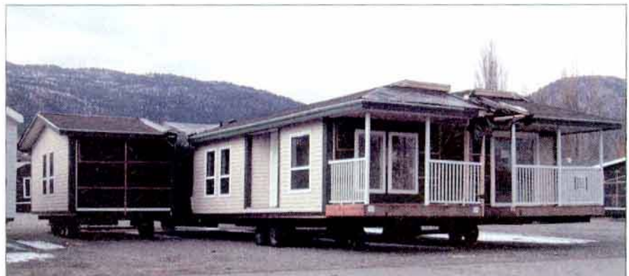
A Landmark double-section, with a pod (called a tag in Canada), a master bedroom and closet addition of 22' long by 11'6" wide, heading to Langley, BC.
